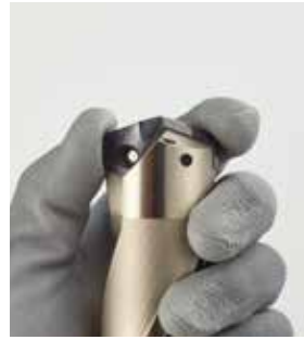
③ Lightly press the insert while screwing to prevent it from rotating.
